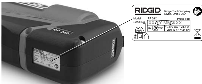
Figure 2 – Machine Serial Number - Circled digits indicate the year and month of the manufacture. (YY = year, MM = month).
